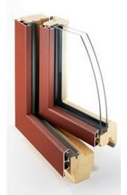
Figure 2: The outer 1-3mm of the Timber profile contains impregnation product, which is covered by a Topcoat of 100-150 µm Source of pictures: Wertbau GmbH
