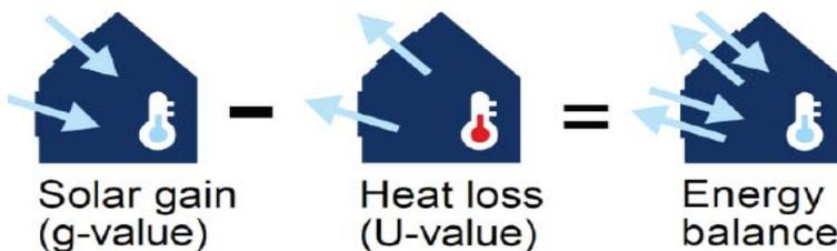
Windows provide free solar gains to buildings in addition to their insulation properties
